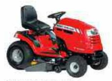
MF 42-20SD 20HP Kohler® V-Twin engine, hydrostatic transmission and ± 107cm (42") side discharge deck.
