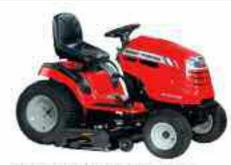
MF 50-235D 23HP\* Kohler®V-Twin ungine, hydrostatic transmission and a 127cm (50") side discharge deck.
