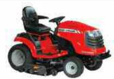
MF 21-22GC 22HP™ Kohler® V-Twin engine, cast-iron hydrostatic transmission and a 127cm (50") side discharge deck.
